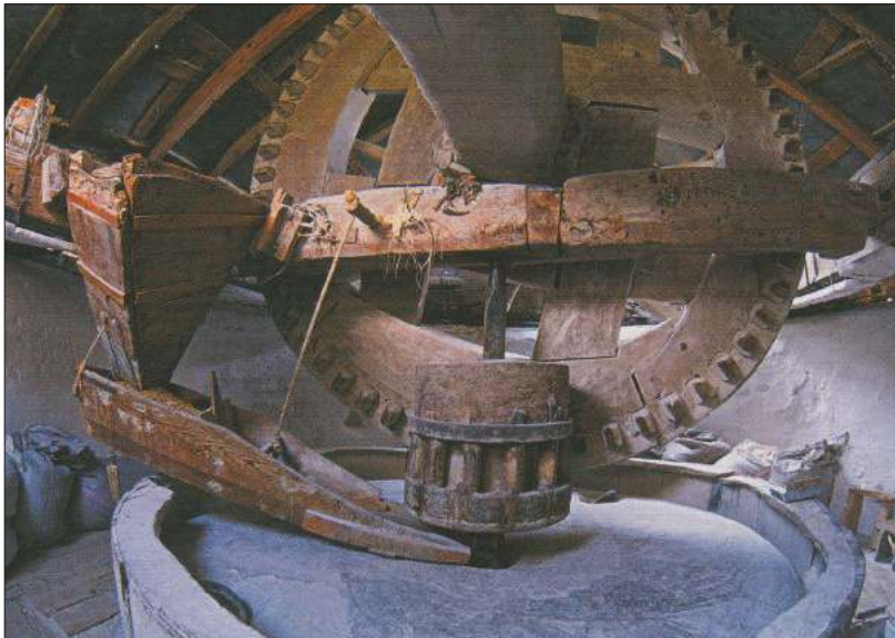
Figure 4. A windmill's cogwheel and cereal shovel on the island Kalymnos (author's pic. archive).
